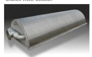
For shallow water conditions, Hendrick offers a patented halfbarrel intake screen. With the same flow characteristics of our T-Intake screens, the bottom discharge outlet allows complete functionality in low water. Ideal for small creeks or rivers where a full T-Intake screen won't work.
